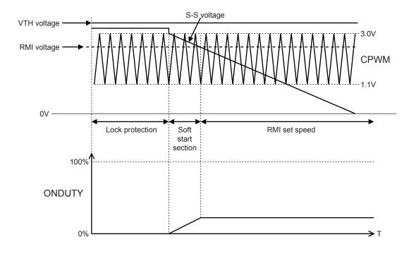
Adjust the S-S pin voltage gradient by means of the capacitance of the capacitor between the S-S pin and 5VREG. Recommended capacitor:  $0.1\mu$  to  $1\mu$ F
